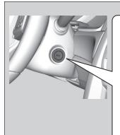
O LOCK: Insert and remove the key in this position.
