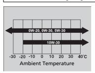
Use a Genuine Honda Motor oil or another commercial engine oil of suitable viscosity for the ambient temperature as shown.
