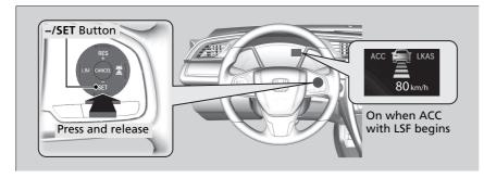
When driving at about 30 km/h (18 mph) or above: Take your foot off the pedal and press the **-/SET** button when you reach the desired speed. The moment you release the button, the set speed is fixed, and ACC with LSF begins.
