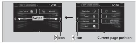
Selecting  $\langle\!\langle\!\langle$  or  $\rangle\!\rangle\!\rangle$ , or swiping the screen left or right changes to the next screen.
