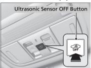
To turn off the ultrasonic sensor system, press the ultrasonic sensor OFF button after you remove the key from the ignition switch, or with the key in the ACCESSORY I or LOCK
