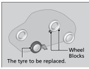
**6.** Place a wheel block or rock in front and rear of the wheel diagonal to the flat tyre.
