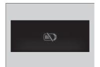
Warning buzzers may sound from inside and/ or outside the vehicle to remind you that the keyless remote is out of the vehicle. If the buzzer continues even after the remote is put back inside, place it to be within its operational range.
