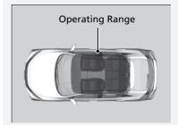
You can start the engine when the keyless remote is inside the vehicle.
