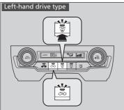
Pressing the (windscreen demister) button automatically switches the system to fresh air mode.
