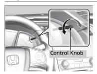
When the position lights are turned on and the ignition switch is in ON [II]\*1, you can use the brightness control knob to adjust instrument panel brightness.
