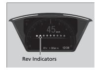
Light up from left to right according to engine speed.
