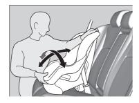
Make sure the child restraint system is firmly secured by rocking it forward and back, and side to side; little movement should be felt.
