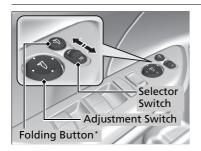
You can adjust the door mirrors when the ignition switch is in ON  $[II]^{*1}$ .
