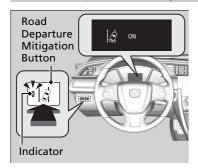
Press the Road Departure Mitigation button to turn the system on and off.
