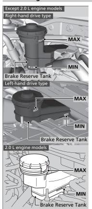
The fluid level should be between the MIN and **MAX** marks on the side of the reserve tank.
