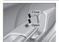
**To open:** Push the switch down. To close: Pull the switch up.
