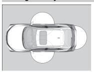
When you carry the keyless remote, you can lock/unlock the doors and hatch.
