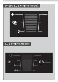
When the turbo charger is producing boost, this meter shows the boost pressure.
