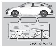
**1.** Place the jack under the jacking point closest to the tyre to be changed.
