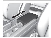
The console lid can be used as an armrest. **To adjust:**Slide the armrest to desired position.
