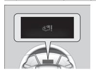
■ When the power mode is set to ON A system warning message appears on the driver information interface if there is a potential problem with the pop-up hood system.
