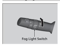
■ To turn the front fog lights on Rotate the switch to the \*\*D. The \*\*D indicator comes on.
