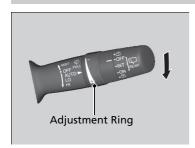
When you push the lever down to **AUTO**, the windscreen wipers sweep once, and go into the automatic mode.
