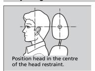
Front head restraints are most effective for protection against whiplash and other rearimpact crash injuries when the centre of the back of the occupant's head rests against the centre of the restraint. The tops of the occupant's ears should be level with the centre height of the restraint.
