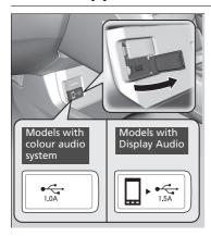
Install the device USB connector or the USB flash drive to the USB port.
