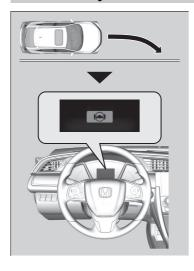
The front camera behind the rearview mirror monitors left and right lane markings (in white or yellow). If your vehicle is getting too close to detected lane markings without a turn signal activated, the system, in addition to a visual alert, applies steering torque and alerts you with rapid vibrations on the steering wheel, to help you remain within the detected lane.
