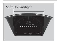
Blinks when the tachometer reading approaches the red zone.
