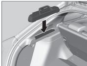
The housing can be installed on either side of the luggage area.
