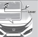
**3.** Pull up the bonnet latch lever (located under the front edge of the bonnet to the centre) and raise the bonnet. Once you have raised the bonnet slightly, you can release the lever.
