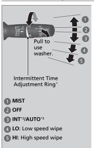
The windscreen wipers and washers can be used when the ignition switch is in ON  $III^{*1}$ .
