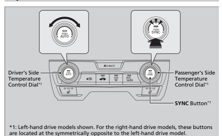
You can set the temperature synchronously for the driver's side and the passenger's side in synchronization mode.
