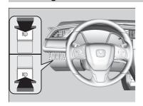
Turn the headlights on and press the headlight washer button to operate. The headlight washers also operate when you turn the windscreen washers for the first time after the ignition switch is in ON  $\boxed{II}^{*1}$ .
