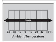
Use a Genuine Honda Motor oil or another commercial engine oil of suitable viscosity for the ambient temperature as shown.
