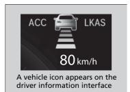
When a vehicle whose speed is slower than your set speed comes in or cuts in front of you and is detected by the radar and the camera, your vehicle starts to slow down.
