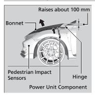
When the pedestrian impact sensors detect a certain amount of impact, the pop-up hood system is activated and the rear of the bonnet will raise.
