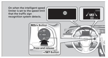
• The moment you release the **-/SET** button or **RES/+** button, the intelligent speed limiter is set to the speed limit that the traffic sign recognition system detects. The speed limit is displayed.
