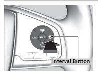
Press the (interval) button to change ACC following-interval.
