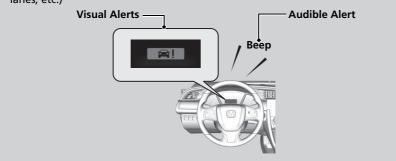
At system's earliest collision alert stage, you can change the distance (Far/Normal/ Near) between vehicles at which alerts will come on through driver information interface or audio/information screen setting options.
