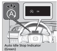
The engine then restarts once the vehicle is about to move again, or depending on environmental and vehicle conditions, and the indicator (green) goes off.
