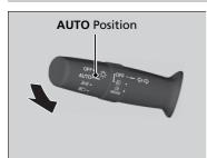
Adjust the system when the vehicle is parked with the ignition switch in ON [II]\*1 and the light switch is in the **AUTO** position.
