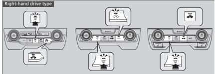
Pressing the (windscreen demister) button turns the air conditioning system on and automatically switches the system to fresh air mode.
