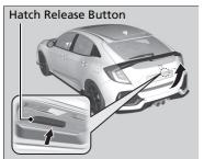
When all the doors are unlocked or press the hatch unlock button on the remote transmitter, the hatch is unlocked. Press the hatch release button and lift open the hatch.
