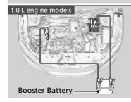
**4.** Connect the second jumper cable to the booster battery
