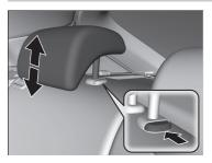
A passenger sitting in a outer back seating position should adjust the height of their head restraint to an appropriate position before the vehicle begins moving.
