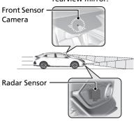
The radar sensor is in the lower bumper next to the fog light\*.
