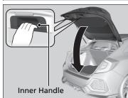
To close the hatch, grab the inner handle, pull the hatch down, and push it closed from outside.
