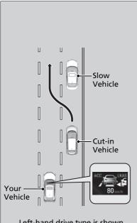
The radar sensor in the lower bumper next to the fog light\* detects vehicles ahead of you including those in the adjacent lane, and the camera behind the rearview mirror detects the lane markings.
