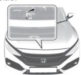
When finished, close the bonnet and make sure it is firmly locked in place.
