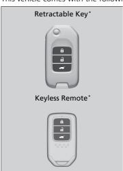
Use the keys to start and stop the engine, and to lock and unlock all the doors and hatch. You can also use the remote transmitter to lock and unlock all the doors and hatch.
